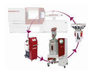
In-line recycling made easy: with Smart Recycling, WITTMANN offers precisely coordinated system solutions from a single source. (Picture: WITTMANN)
